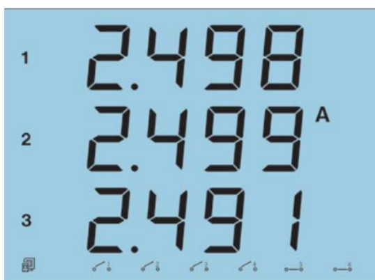
Fig 3.4 Three phase current
