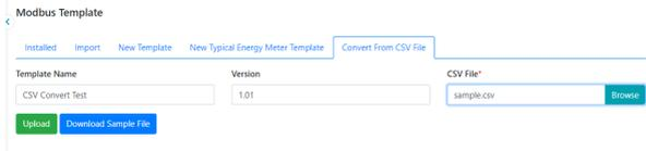
Figure 5-13 AcuLink 810 Convert Modbus Templates from CSV File
