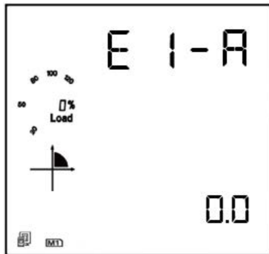
Figure 3-19 Energy 1 (To Generator) Display
